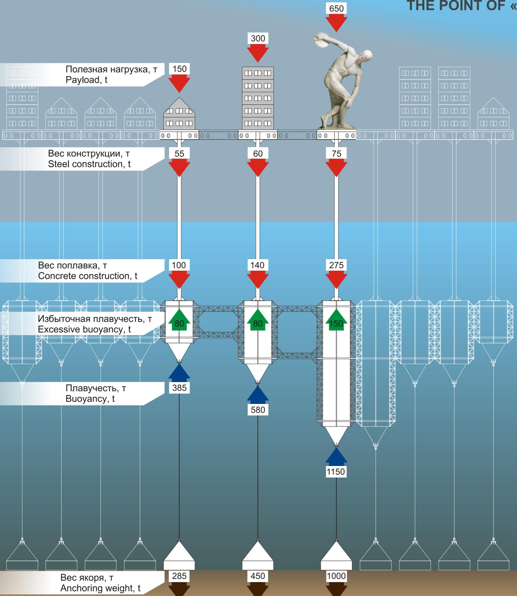
For constructing structures on 'tension legs', a complex of underwater floatages is used. On each floatage acts hydrostatic buoyancy force, which is fixed by a flexible interlinking with the anchor, laid on the seabed. Thus, all the floatages are hanging in the water at a certain distance from the water surface.
